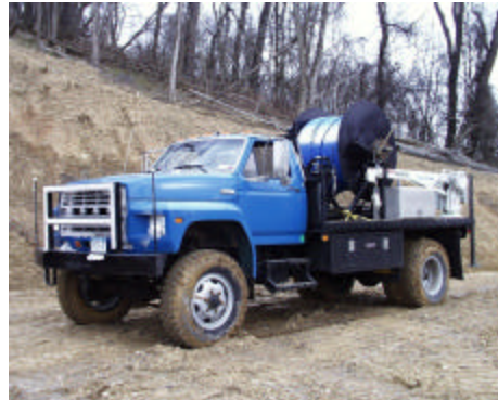
Fig. 2 Direct drive Spooling Truck
