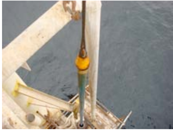
Figure 5: Tubing coming through the riser
